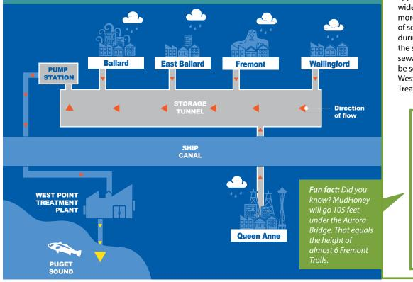
long, running from Ballard to Wallingford, and approximately 18-ft, 10-in wide. It will temporarily hold more than 29 million gallons of sewage and stormwater during heavy rains. When the storm passes, the stored sewage and stormwater will be sent to King County's West Point Wastewater Treatment Plant.
