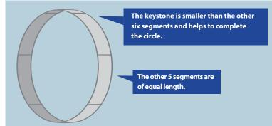
\*This is a graphic representation of a ring and is not an exact replica of what will be built by MudHoney.
