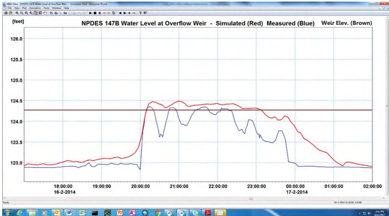
Figure 5-17: Water Level at NPDES 147B Overflow Weir – Fourth Largest Overflow Volume Event 2011-2015
