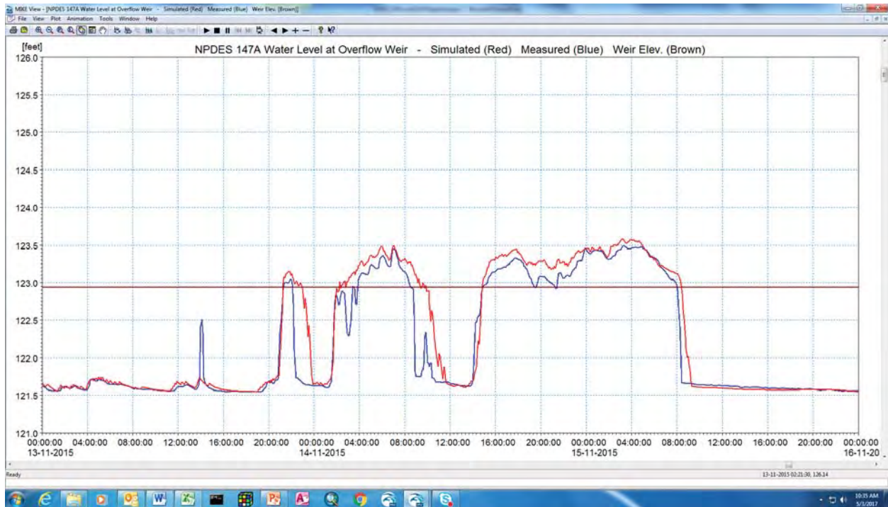
Figure 5-8: Water Level at Overflow Structure 147A - 5th Largest Simulated and Measured Overflow Volume Event
